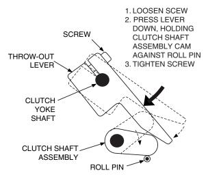
Figure 7: Drive Clutch Adjustment
