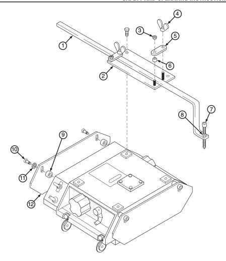
Figure 15: Radius Rod Assembly (top), Part No. 0252-0040 Heat Shield (bottom), Part No. 0252-0103
