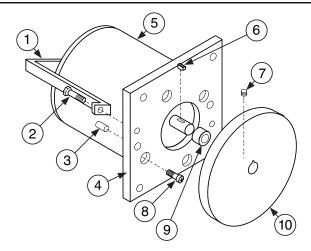
Detail C: Motor Disk Assembly, Part No. 0252-0132 / 0252-0142 VCM-200HT
