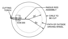
Example 2: The cutting torch position outside the path of the cutting machine.
