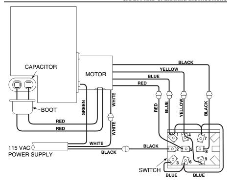
Figure 8: Pictorial Wiring Diagram, VCM-200
