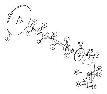
Detail A: Cone Disk Assembly, Part No. 0252-0129
