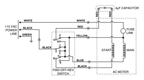
Figure 9: Schematic Wiring Diagram, VCM-200
