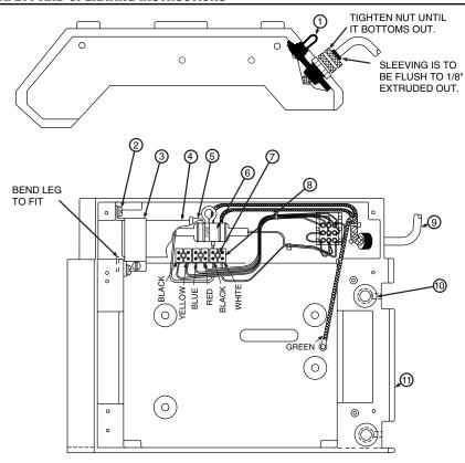
Figure 16: VCM-200HT Outer Case Assembly, Part No. 0252-0116
