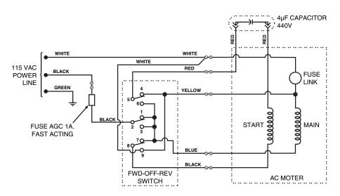
Figure 11: Schematic Wiring Diagram, VCM-200HT (Hi-Temp)
