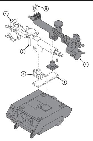
Figure 3: Setup with Dual Torch Mount
