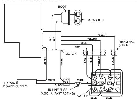
Figure 10: Pictorial Wiring Diagram, VCM-200HT (Hi-Temp)
