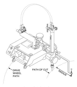
Figure 5: Circle Cutting Setup
