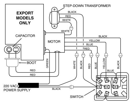
Figure 18: Pictorial Wiring Diagram, VCM-200E
