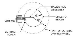
Example 1: The cutting torch positioned inside the path of the cutting machine.
