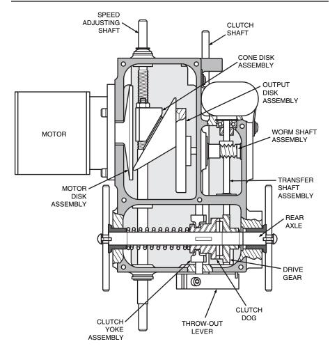
Figure 6: VCM-200/VCM-200HT/VCM-200HS Internal Assemblies
