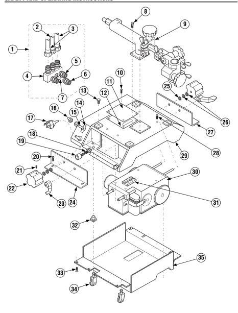
Figure 13: VCM-200 / VCM-200HT\* Series Main Assembly (\*For continuous use at up to 300°F)
