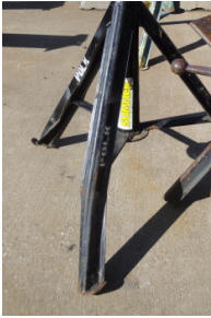
Damaged / Bent Legs
