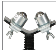
Standard Vee Head Ball Transfer Set Part # 780551 (standard) Part # 780274 (stainless steel) Attachments slide over standard vee head. Accommodates 3/8" - 12" (10 - 300 mm) pipe sizes. 1,000 lb (450 kg) capacity.
