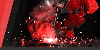
Our gouging carbon electrodes are designed for use in the air carbon-arc metal removal process which melts metal with an electric arc, then blows it away with compressed air. When it's important to save the metal pieces that have been welded together, carbon-arc gouging is an absolute lifesaver!
